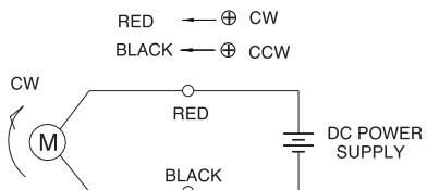
The direction of motor rotation is as viewed from the front shaft end of the motor
